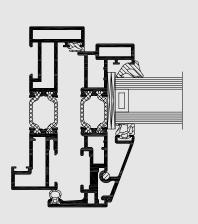
CS 24-SL is a thermally insulated three-chamber window system that combines ultimate elegance with elevated strength and ease in production. The system's slender exterior contours and glazing beads on the outside give the system a steel look design. This slim appearance makes CS 24-SL the ideal system for new-build constructions as well as for the replacement of steel-framed windows, respecting the original design.
